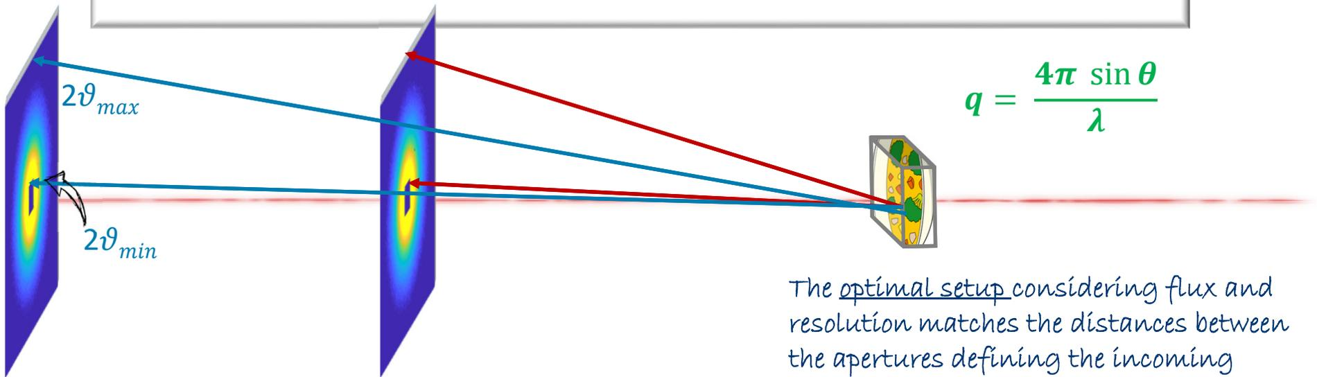
$$\tan 2\vartheta \approx 2\vartheta = \frac{\text{distance pixel to beam centre}}{\text{detector distance}}$$
