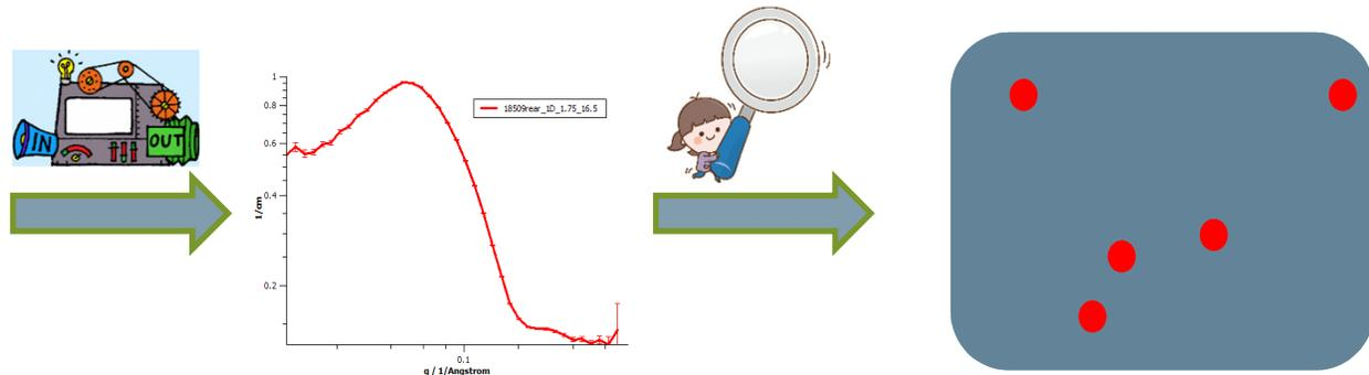
$$I(\theta, \lambda) = I_0(\lambda) \cdot \frac{\partial \Sigma(q)}{\partial \Omega} \cdot \Delta \Omega \cdot t \cdot T(\lambda) \cdot \eta(\lambda)$$
