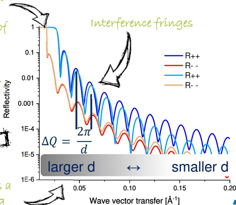
The magnetic potential is determined by dipolar interaction between neutron magnetic moment and moments in the magnetic layer. Can be described by a magnetic scattering length density.
