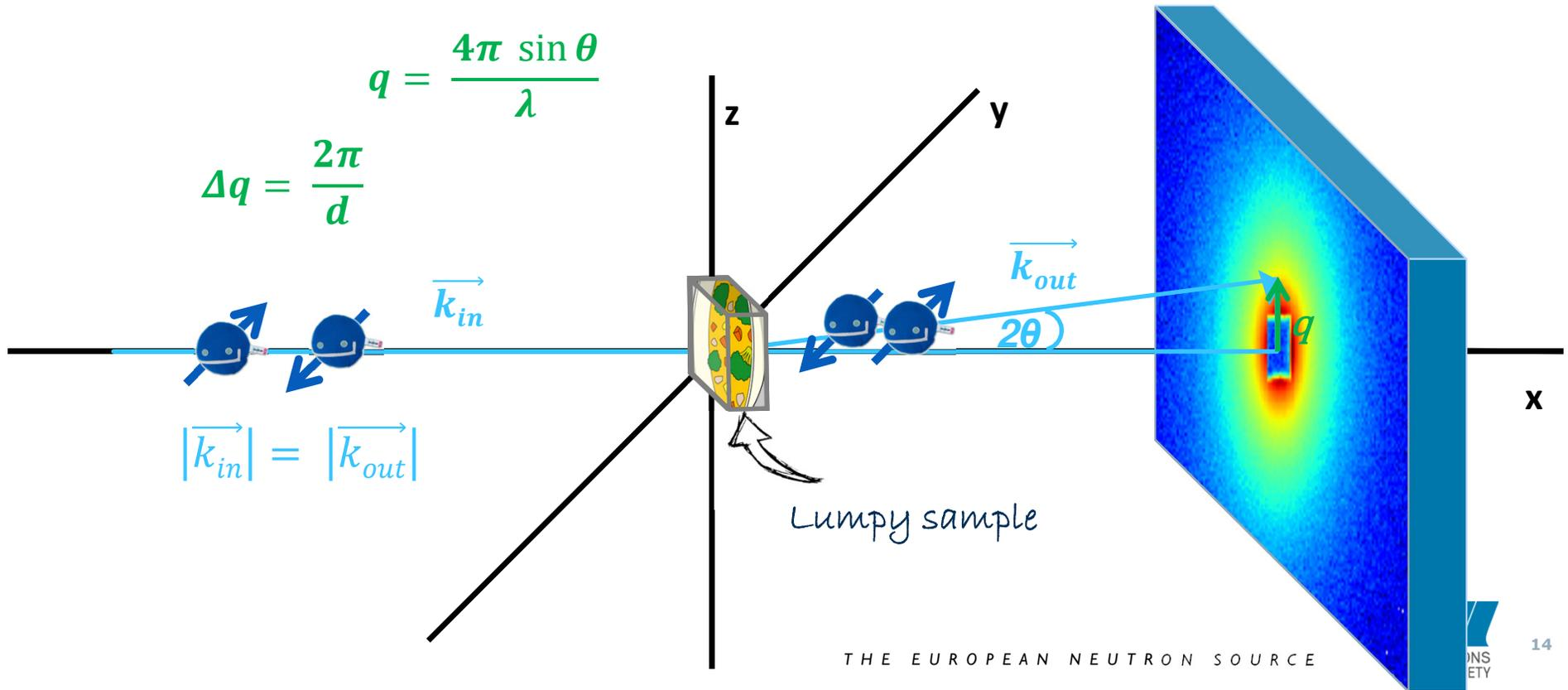
The principles of elastic (neutron) scattering apply also to small angle (neutron) scattering.
