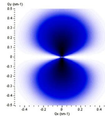
$$\frac{d\Sigma_{mag}}{d\Omega}(q, B_{ext}) = \frac{X}{V} (\Delta\rho_m V_p)^2 \langle \sin^2\phi \rangle P(q)$$
