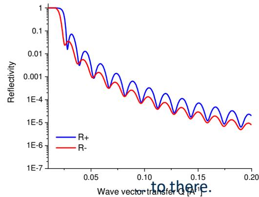
Reflectivity is neutron interference from thin layers.
