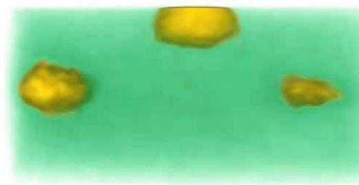
Flux pinning at cooling down below  $T_c$  while applying a homogenous magnetic field of 10 mT perpendicular to the beam.
