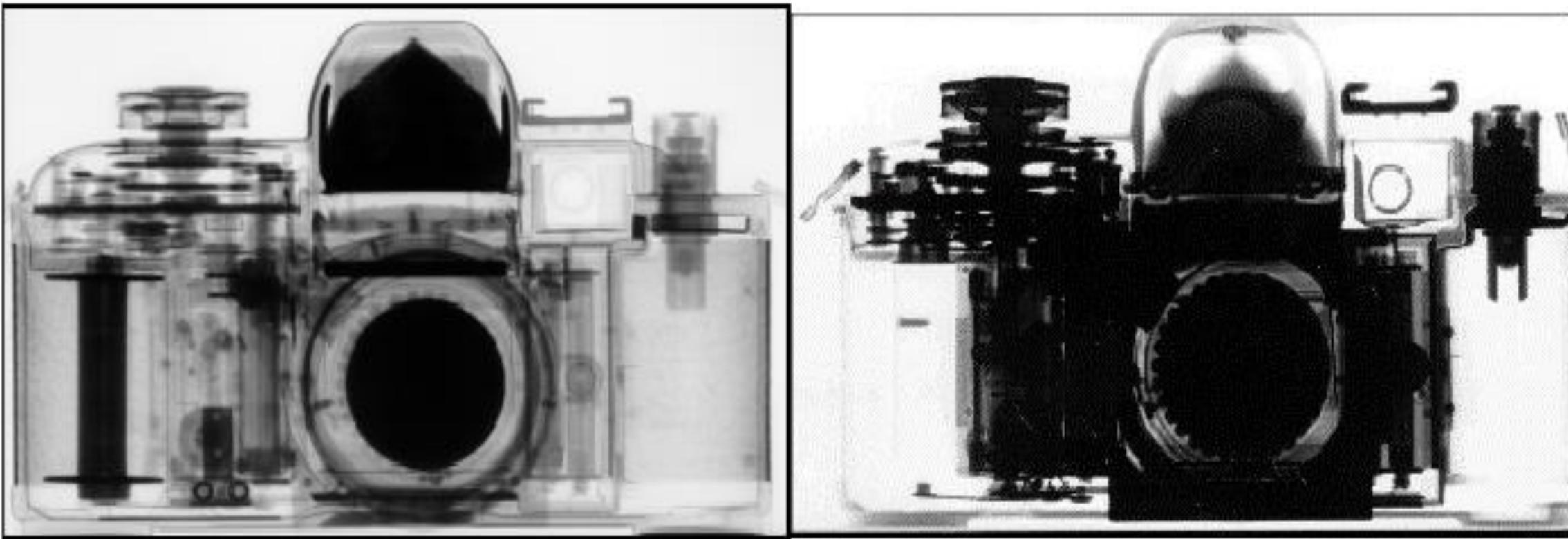
Complementary radiography of a camera using neutrons (left) and X-rays (right). Whereas the hydrogen containing parts can be visualised with neutron even at thin layers, thicker metallic components are hard to penetrate with X-rays.
