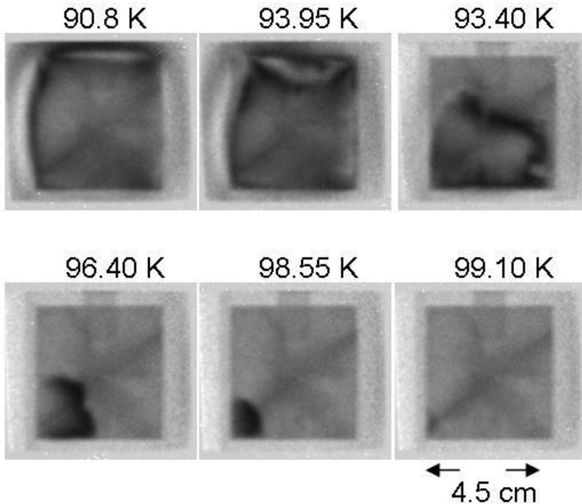
Flux trapping in a 45x45x12 mm<sup>2</sup> bulk YBCO sample.
