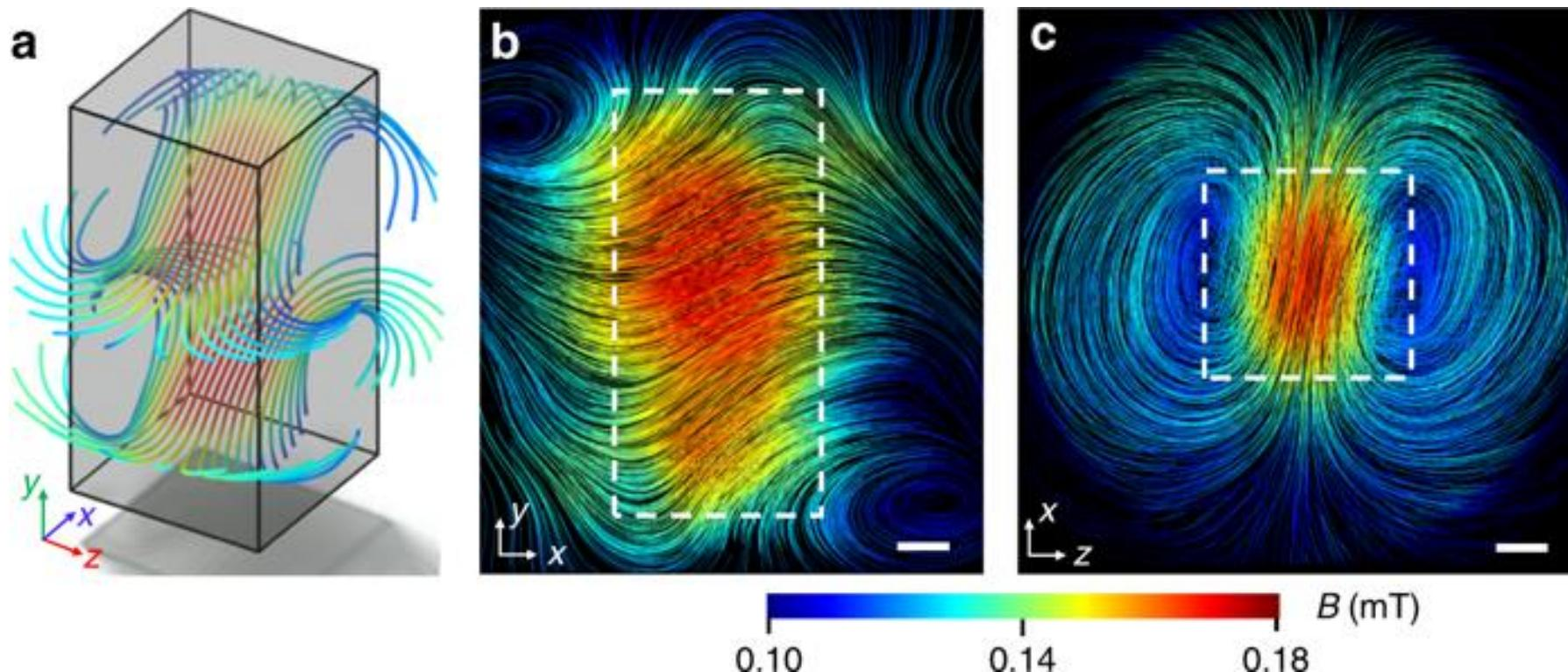
Magnetic vector field inside a superconducting lead sample measured at  $T = 4.3$  K. a Some selected magnetic field lines show the location of the magnetic field inside the sample indicated by the cuboid. b Magnetic field lines in a selected  $xy$  plane (silhouette of the lead sample marked by dotted lines). Scale bar, 5 mm. c Magnetic field lines in a selected  $xz$  plane. Scale bar, 5 mm.
