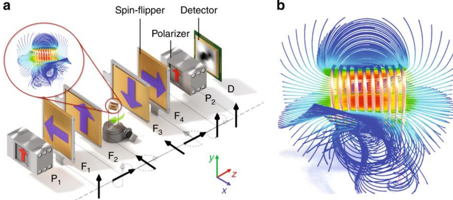
Tensor tomography. a Schematic drawing of the setup used for tensor tomography with spin-polarized neutrons, comprising spin polarizers (P), spin flippers (F) and a detector (D). b Selected magnetic field lines around an electric coil (calculation)
