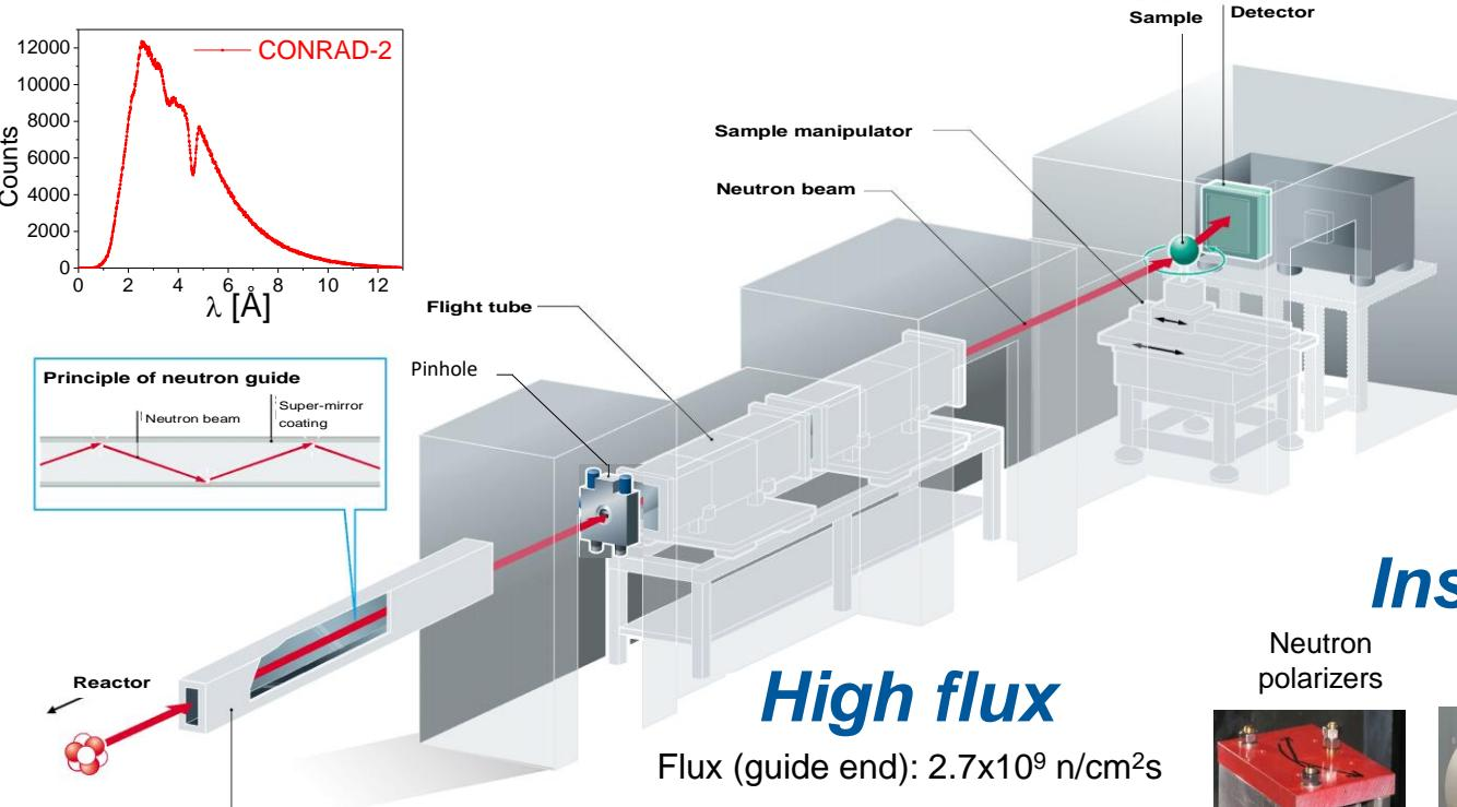
Guide system: super-mirror coated neutron guide (M=3) with a curvature of 750 m and length of 15 m followed by linear guide section (M=2) with a length of 10 m.
