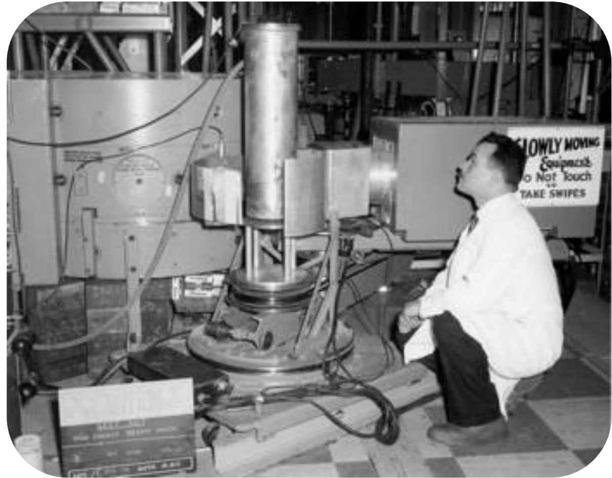
B.N. Brockhouse with the first version of his triple-axis spectrometer at the NRU reactor (November 1958 – July 1959)
