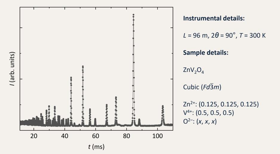
Step 1: Read in the data, instrumental details and crystal structure model
