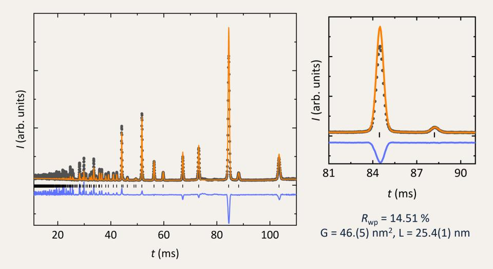
Step 5: Refine the atom positions and thermal displacements
