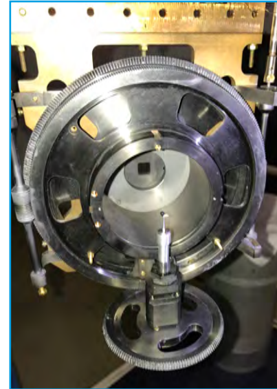
Cryocradle setup allowing for out-of-plane access
