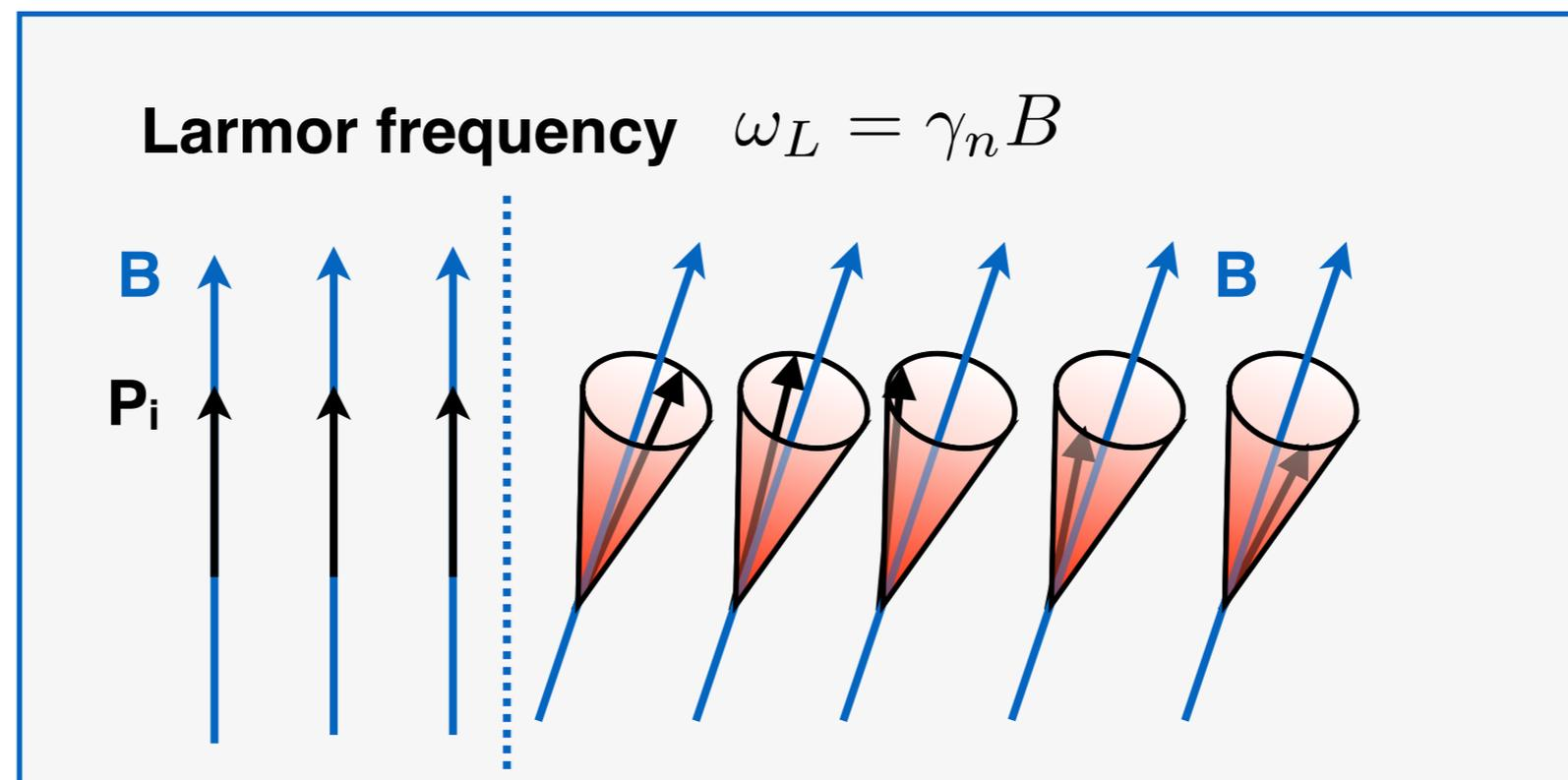
The angle of the cone depends on the angle between the original field direction and the new field direction.
