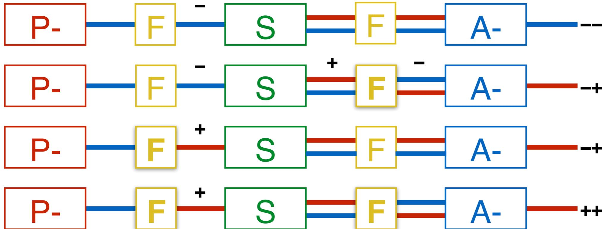
We have also seen that it can be useful to rotate the polarisation versus **Q** and **M** — **guide field**. The guide field also preserves the polarisation between the elements.
