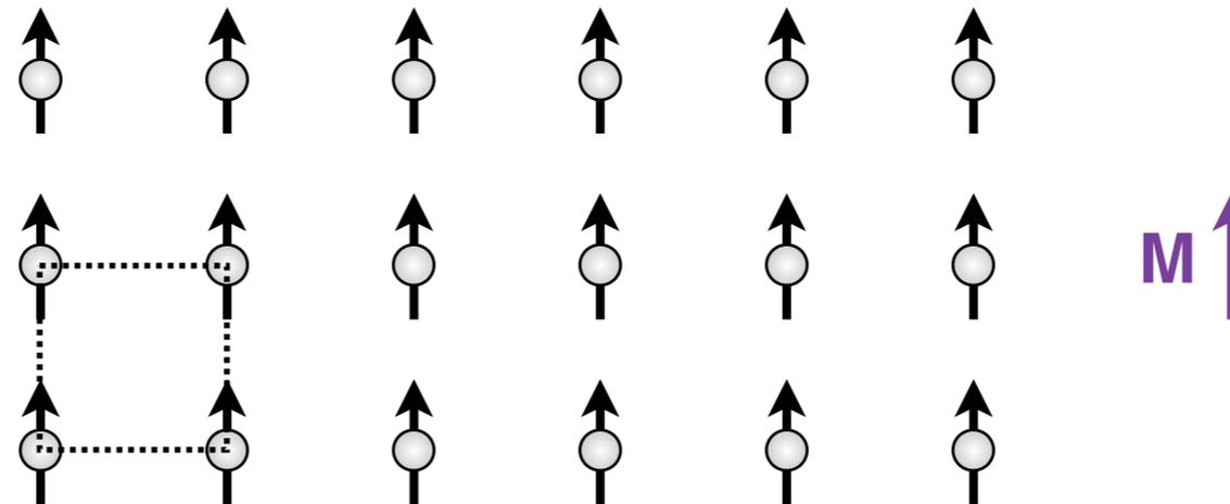
Bragg peak cross section now depends on the orientations of the magnetisation  $\mathbf{M}$ ,  $\mathbf{P}_i$ , and  $\mathbf{Q}$ . It also includes **both** nuclear and magnetic contributions. For  $\mathbf{M} \parallel \mathbf{P}_i \perp \mathbf{Q}$ :
