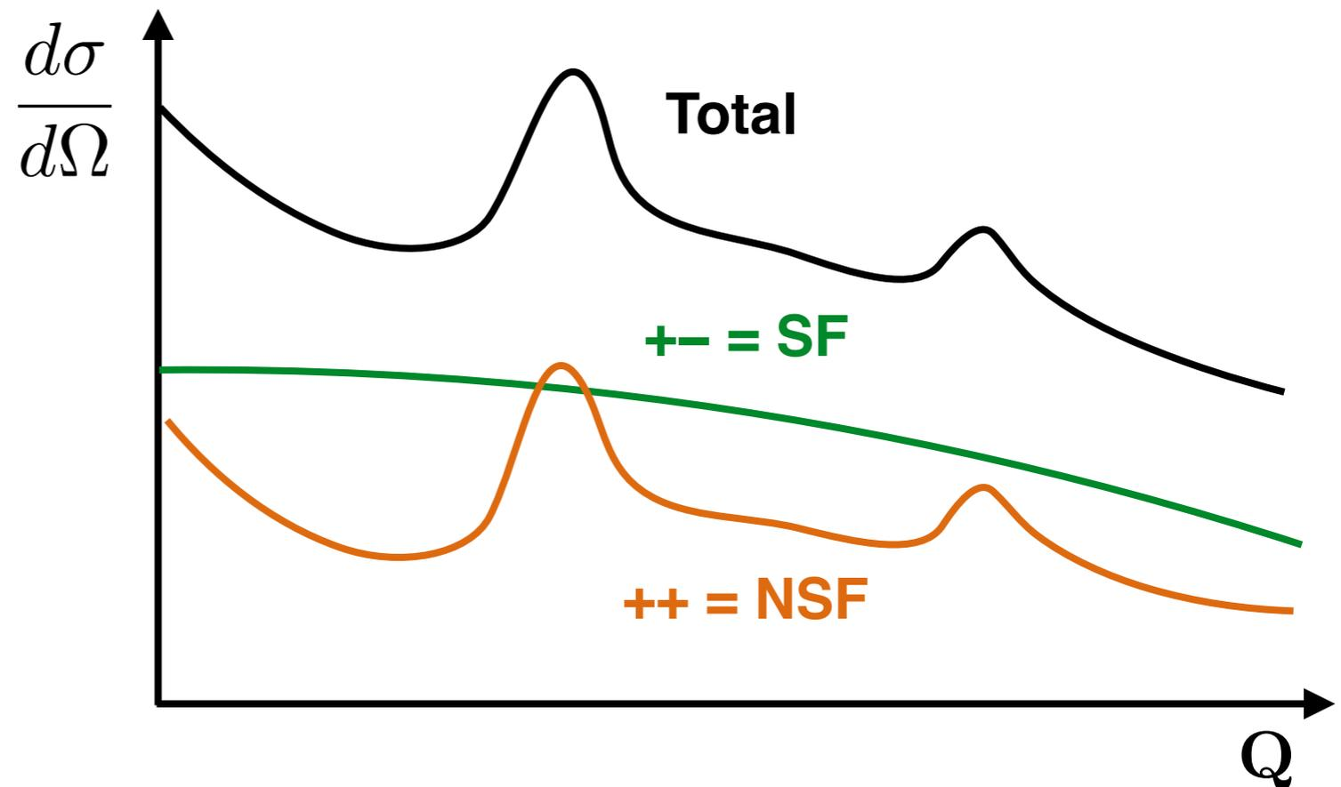
If we perform longitudinal polarization analysis, we can separate the contributions:
