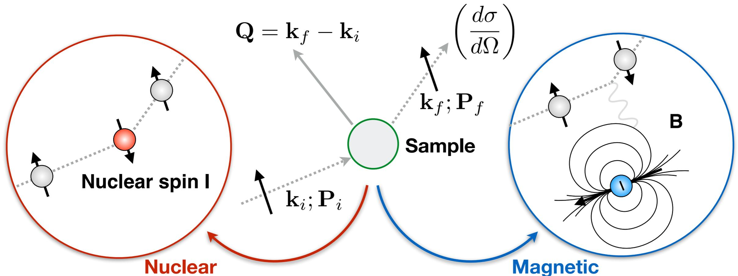
The **scattered polarization** and **cross section** (intensity) depends on the relative orientation of the beam polarization and the magnetic moments in the sample.
