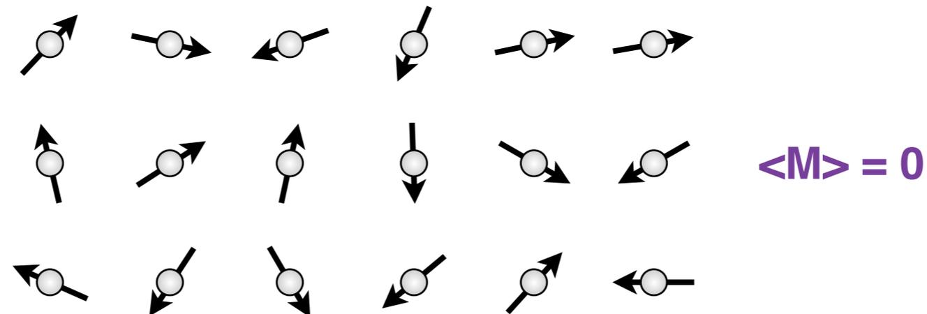
After averaging over the random direction of  $\mathbf{M}$ , the magnetic elastic scattering cross section only depends on angle between the incident polarization  $\mathbf{P}_i$  and  $\mathbf{Q}$ :
