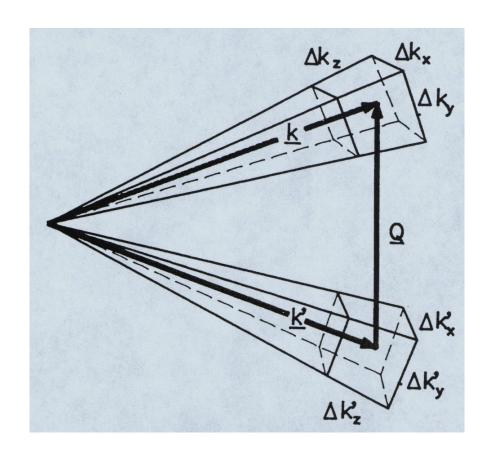
The better the resolution, the smaller the resolution volume and the lower the count rate
