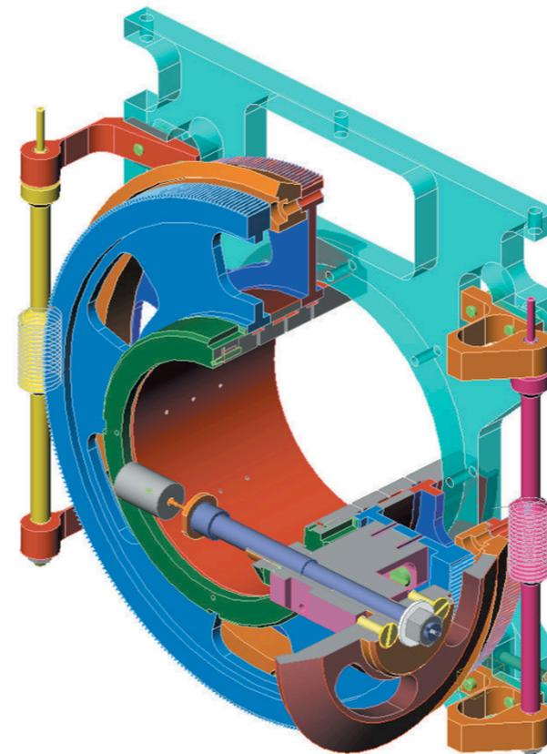
Hot neutron 2-axis diffractometer at the ILL
