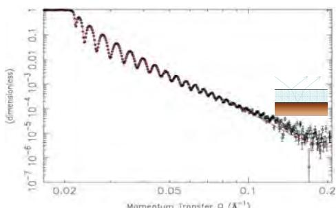
First reflectivity measured on INTER. Nickel/Carbon film (1216 Å) on glass
