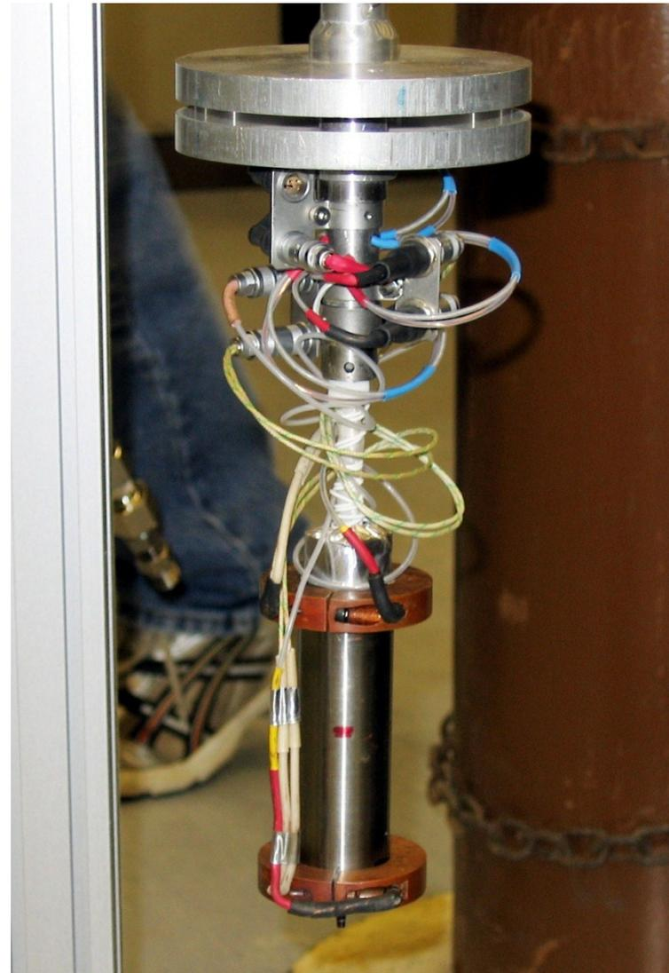
The gas cell design makes a liquid loading unavoidable due to embrittlement of the Bridgman seal at low-T
