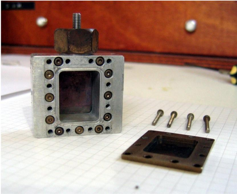
Low temperature studies are made using an aluminium slab can with vanadium windows.
