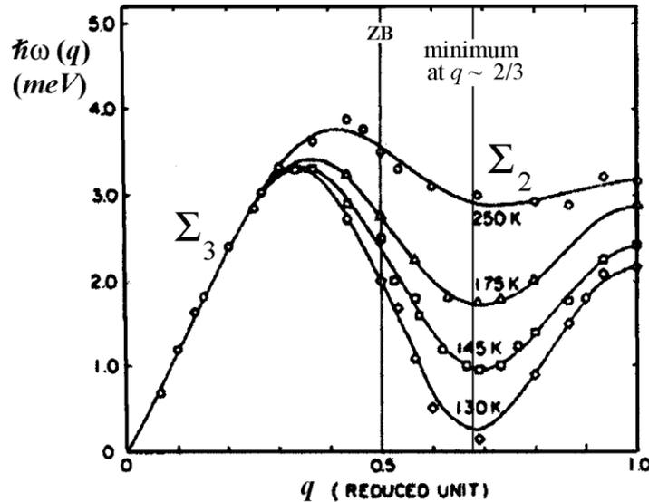
Dispersion relations of the  $\Sigma_2$  soft mode and the  $\Sigma_3$  acoustic mode in  $K_2SeO_4$  plotted in an extended zone. Z.B. indicates the original zone boundary. The solid lines show the results of fitting force constant models to the data.
