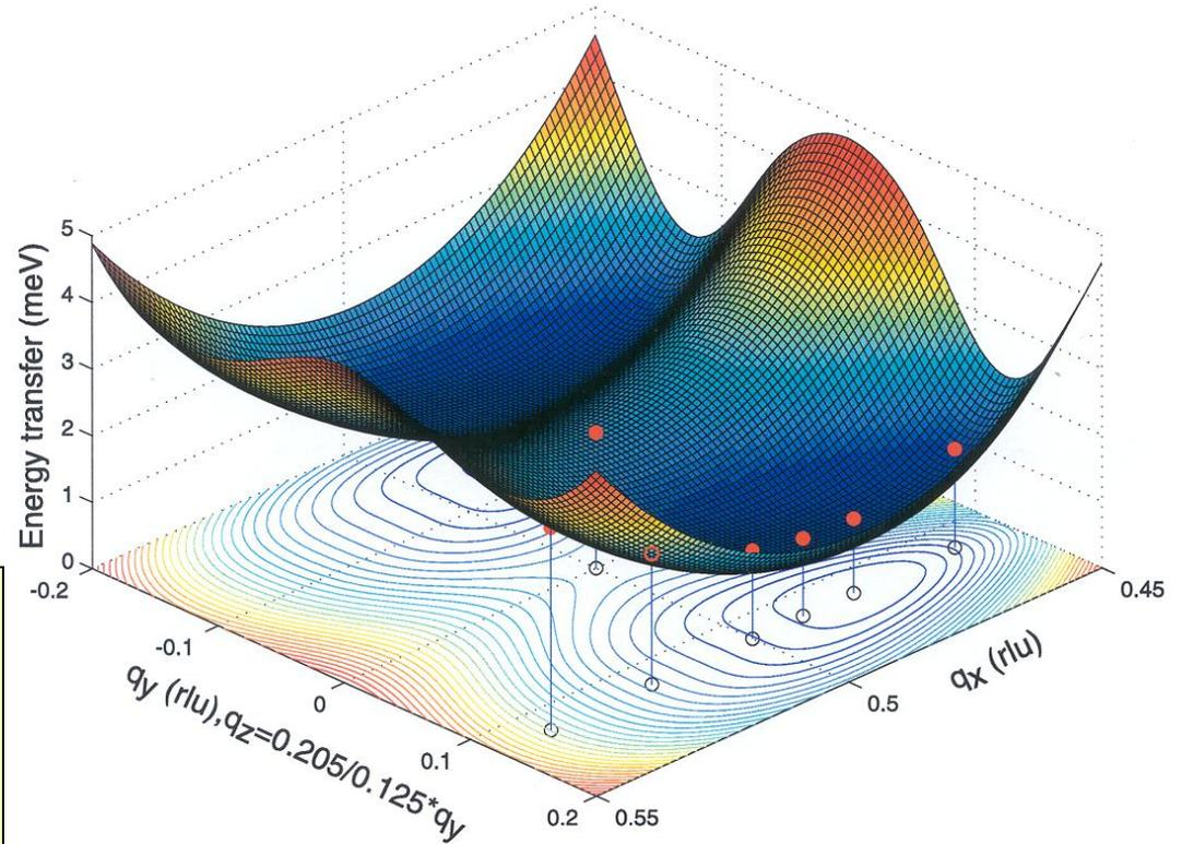
The transition does *not* occur at a high symmetry direction. One needs components along all three crystallographic directions, and none of them are commensurate at  $T_{\text{CDW}}$
