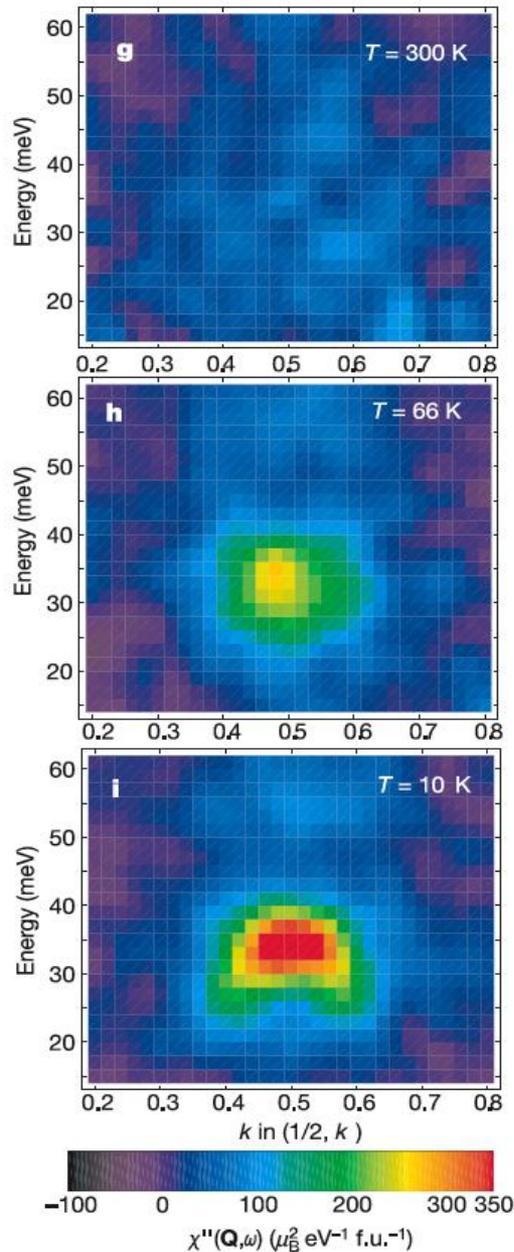
Although there are magnetic excitations over a wide range of energies near  $(1/2, 1/2)$ , they are by far the strongest at the resonant energy, in this case 34 meV, and below  $T_c = 63 \text{ K}$
