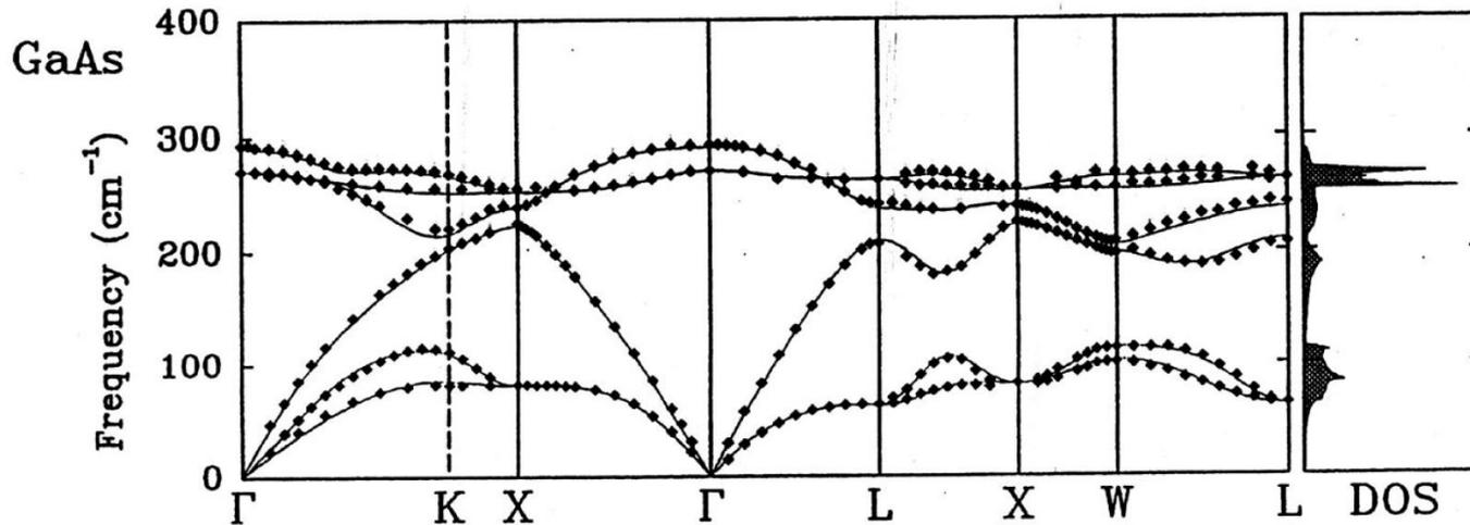
Phonon dispersion curves as measured for GaAs. Strauch & Dorner (1990). The lines give the result of *ab initio* calculations and show that the forces between the atoms are well understood. The letters below give the notation for the symmetry directions or points.
