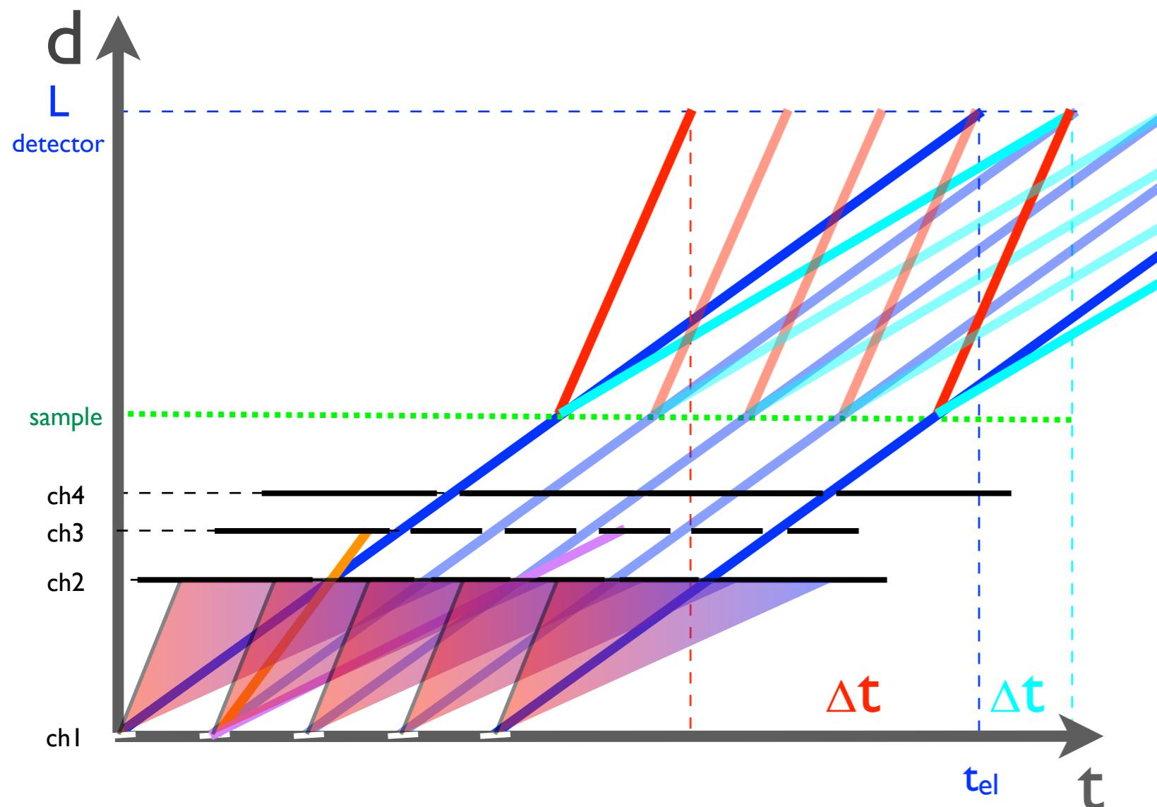
The initial neutron velocity  $v_n^0$  is determined by a multi-chopper system in the primary spectrometer, which transmits monochromatic short pulses with start time  $t_0$  and prevents frame-overlap of scattered neutrons.
