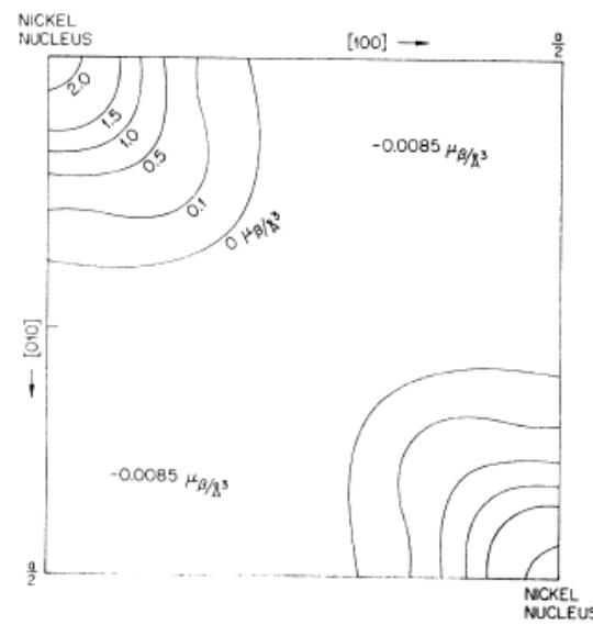
FIG. 4. The magnetic moment distribution in the [100] plane.
